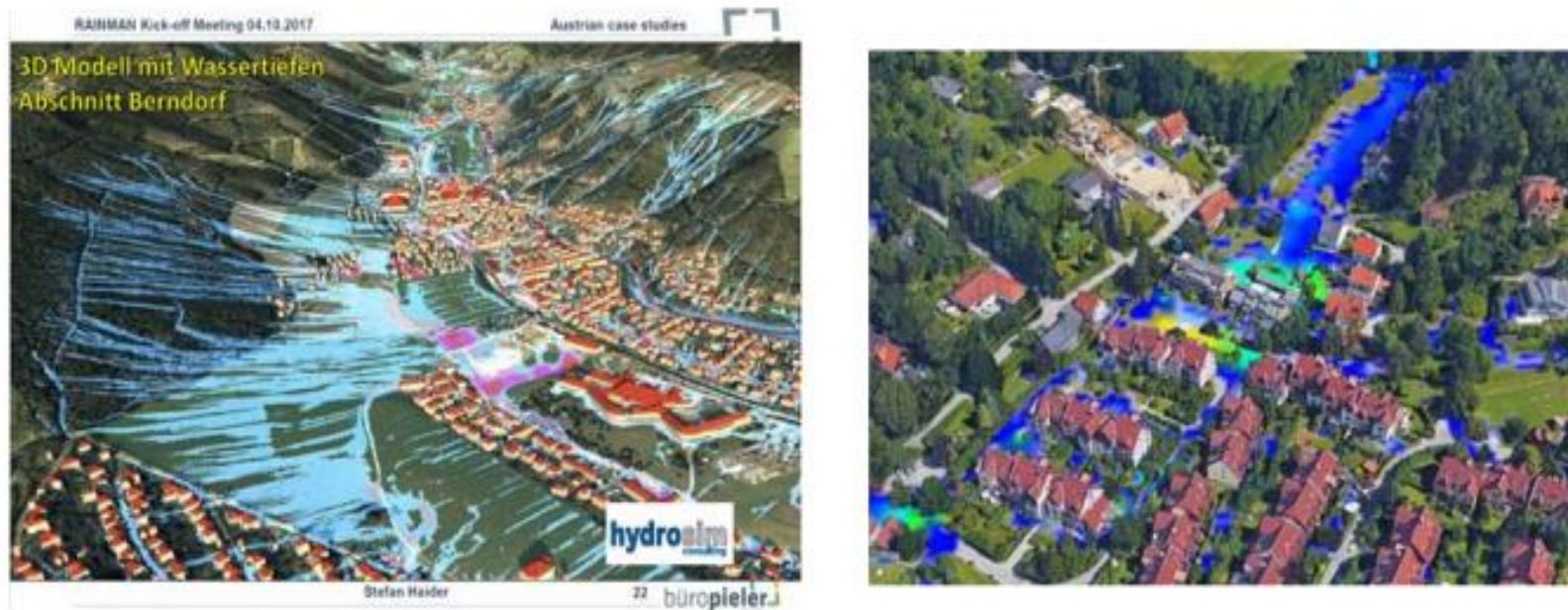
Figure 14: 2D hydrodynamic simulation results (left source: Büro Pieler ZT GmbH and hydrosim consulting, 2014 cited in Haider 2017) (right source: Gamerith et al., 2017)
