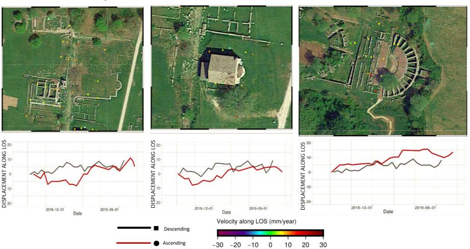
At the Forum-Temples-Church area, during the fall period (Nov 2018 – continuous trend downward. the PS highlights a weak movement Jan 2019), then stable until the end. upward and westward, by 5-10 mm At the Theater the PS show a
