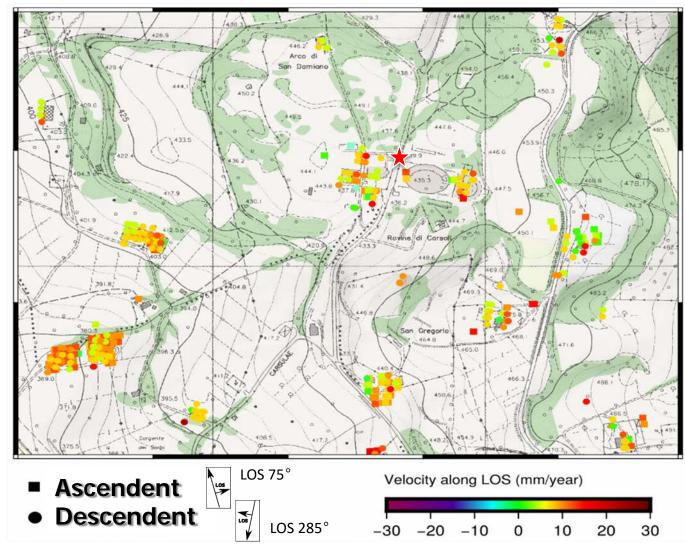
**DInSAR analysis** has been conducted using SAR data from Sentinel-1 to run the SBAS technique.
