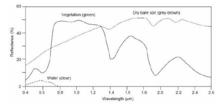
Typical spectral reflectance curves of common earth surface materials in the visible and near to mid-infrared range. Credits: Department of Geology, Aligarh Muslim University, India
